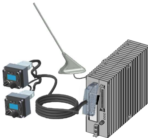
Figure 2: Tandem Application - 2x RCU6512-(3XX) + RT6512 + Antenna (example)
