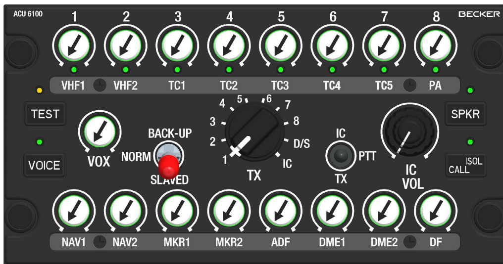
Figure 3-18 Special Version Audio Control Unit ACU6100-X-(XXX0) Intercom /PTT Switch on ACU
