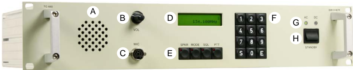
Figure 15: TG660 – Controls and Indications
